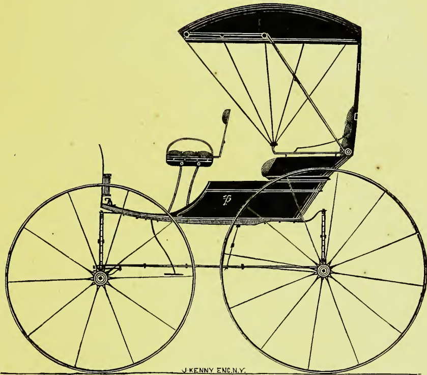
KIMBALL PATENT JUMP-SEAT.— \frac{1}{2} IN. SCALE.
